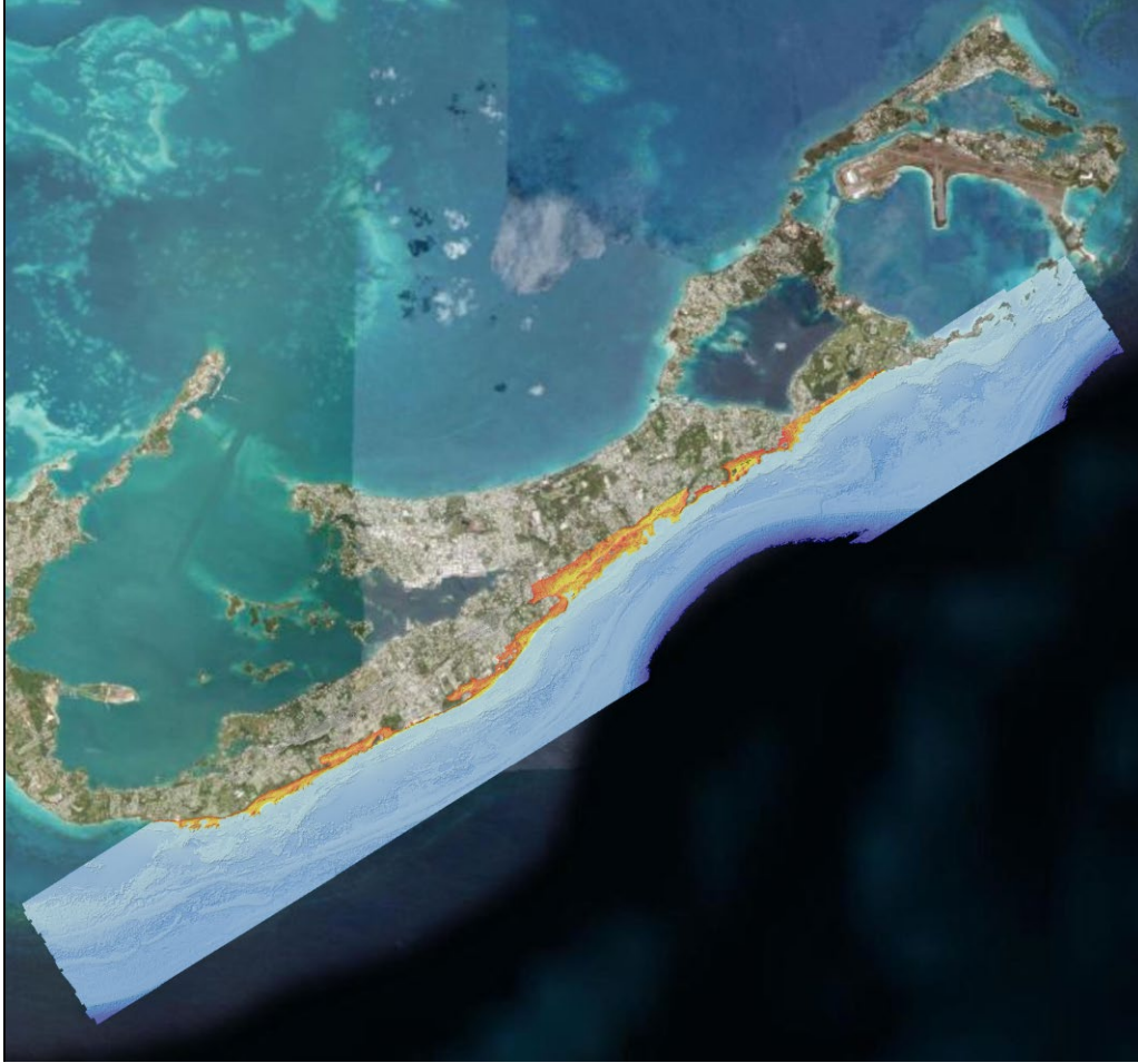
Figure 9.1 2004 lidar coverage of Bermuda; orange and reds are land area data coverage (i.e. the points above sea level) and light blues are bathymetric data coverage
