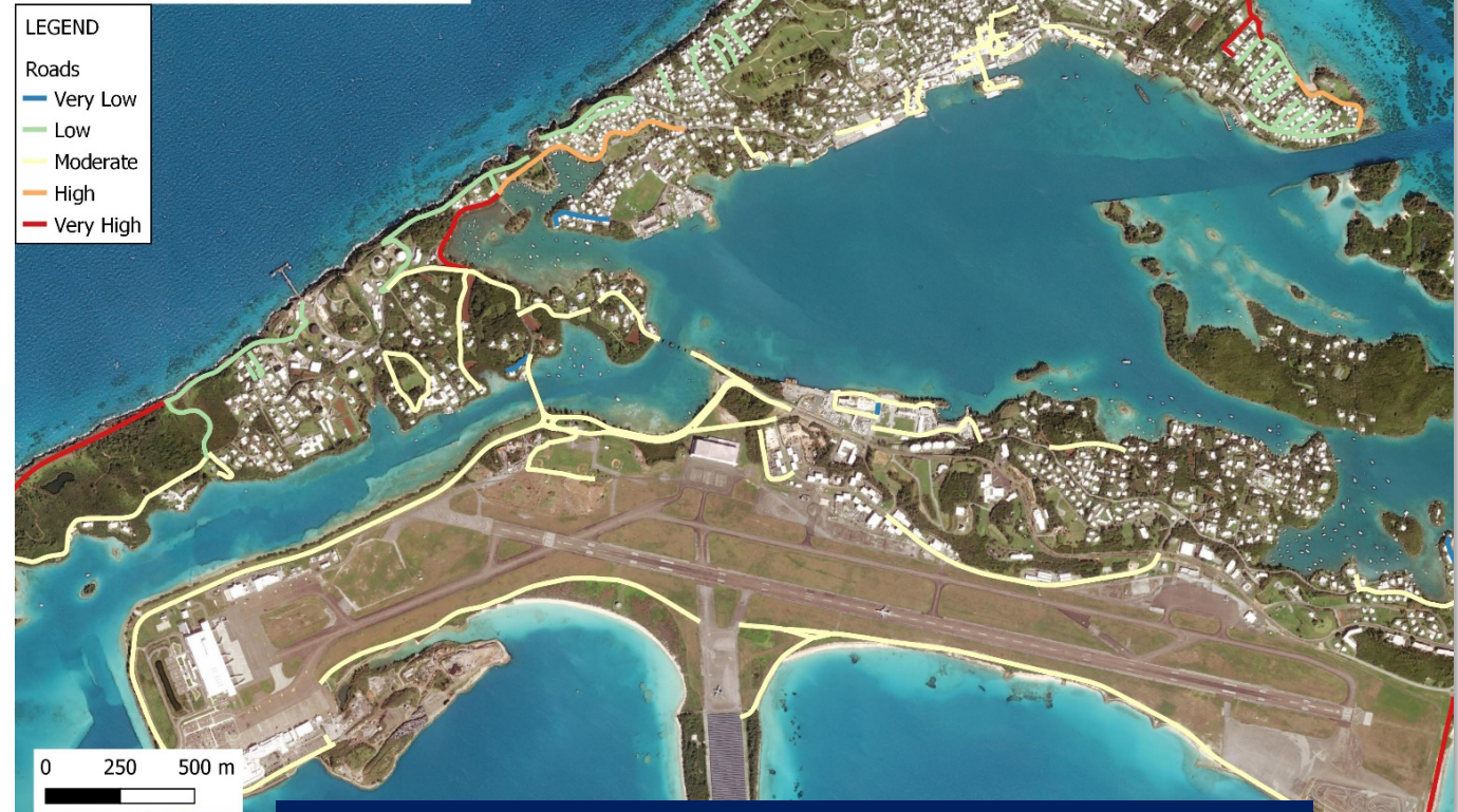
Road vulnerability index for the RCP 8.5, 100-yr horizon, 150-yr event in SMU12
