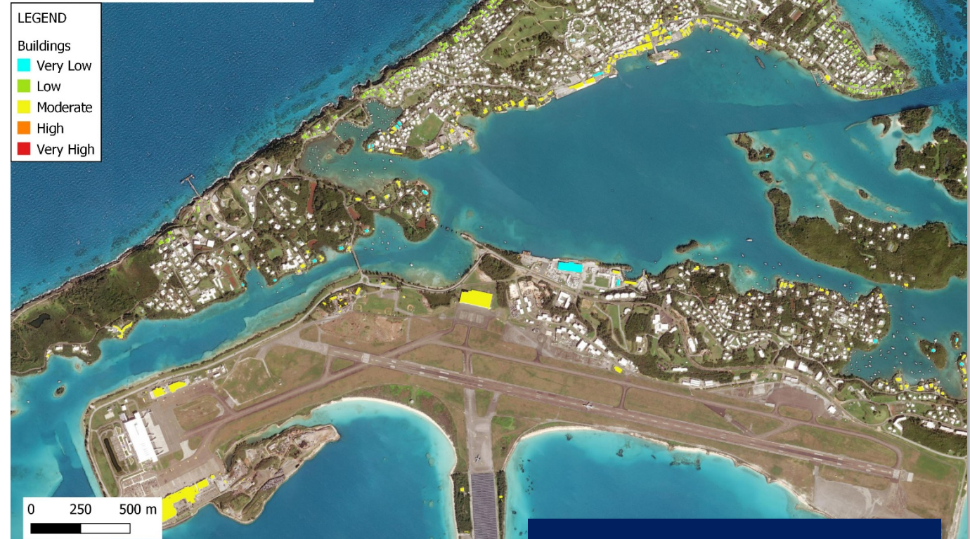
Building vulnerability index for the RCP 8.5, 100-yr Horizon, 150-yr event in SMU12
