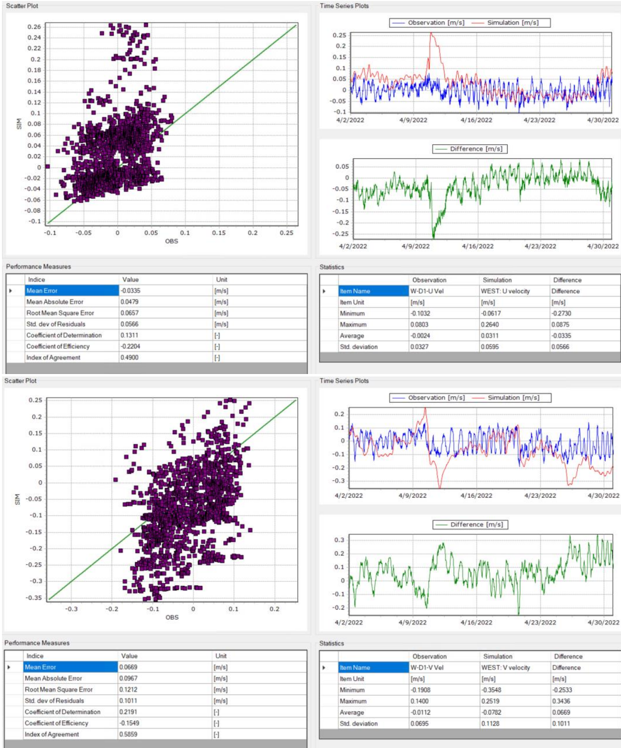
Figure 3.16 ADCP West D1 measured scatter vs modeling scatter u (east-west) and v (north-south) components of the velocities and corresponding progressive vector plot
