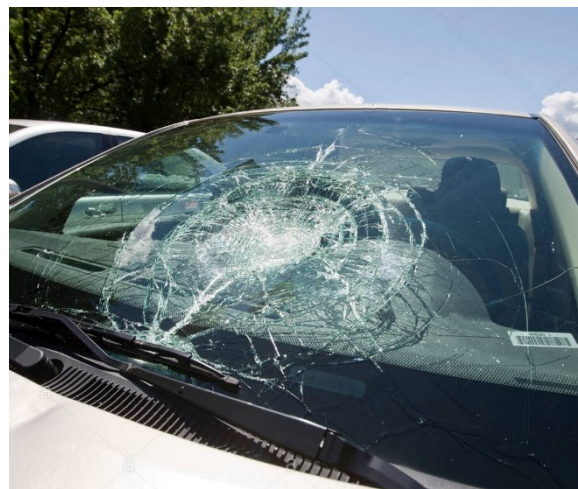
Figure 8: Shattered front windscreen of a car after striking a feral chicken on the road
