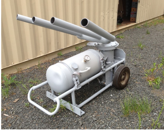
Figure 13: Air powered net launcher
